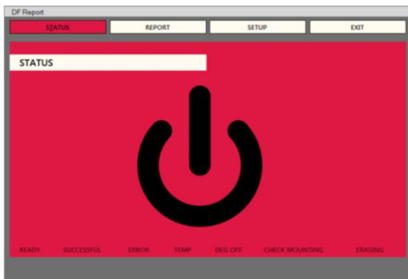
If you have installed the report and certificate kit, optical sensors will identify the status of the degausser and when ready you will use the remote control to start the erase process. The software controls the communication from the degausser through the reporting hardware kit to the reporting control center where the operator can create, save or edit reports. These reports can be printed as a certificate or uploaded to the Blancco Management Console.
